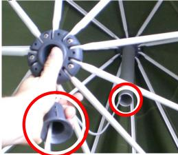
4. Unscrew the two socket screws at the end of the mounting support. To do so you will need two 3mm hex keys. You may find it somewhat difficult to remove the screws, as an adhesive was used to secure them.
