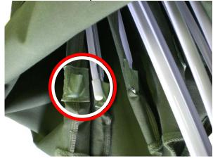
8. Once the canopy covering has been replaced, the rope must be inserted as follows: You will need about 45 cm of strong wire. Bend in the ends of the wire to avoid injury and to form a loop. Fasten the end of the rope to the wire loop as shown in the following illustrations.
