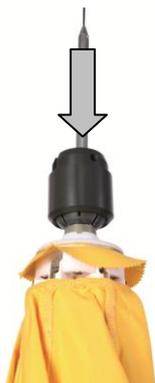
8. Push the hub of the canopy into the cross arm and then turn the canopy 90° (a quarter turn) until the two centring bolts lock into the groove. This ensures that the canopy is tightly connected with the cross arm.
