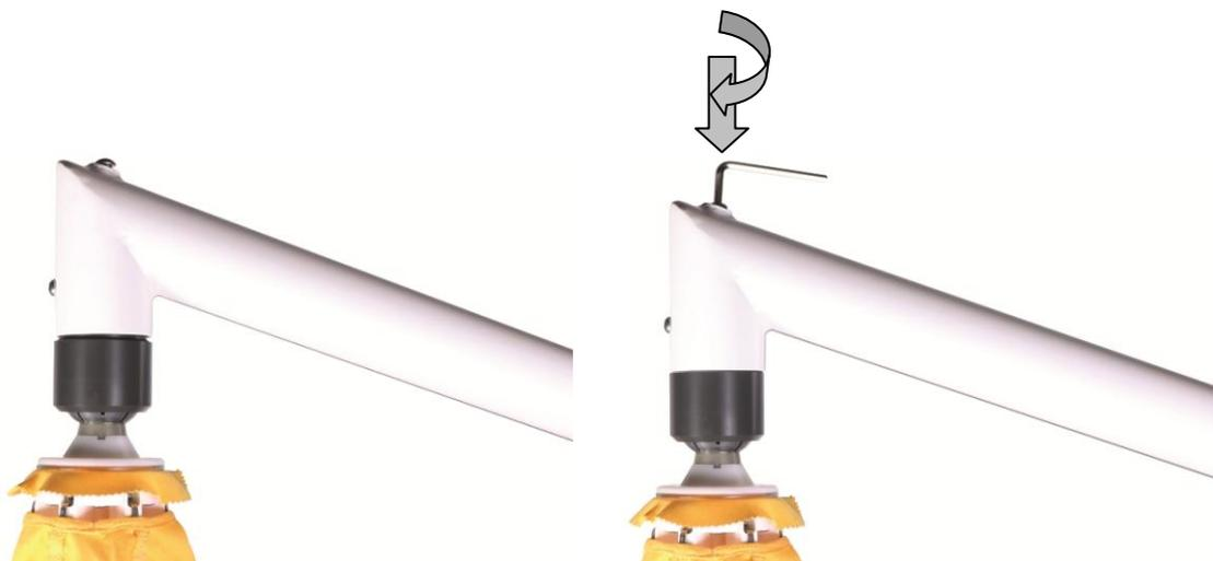
10. Remove the lashing strap of the canopy covering. Open the canopy slightly by gently parting the spokes so that you have access to the inside of the canopy. Use a hexagon key to push the cross bolt out of the ball until limit stop.
